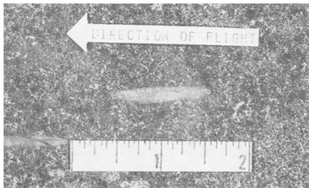
FIG. 2—Comet-shaped scuff mark on the inside of a ricochet mark.
