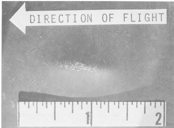
FIG. 1—The exterior of a ricochet dent showing paint fractures that indicate the direction from which the shot came.
